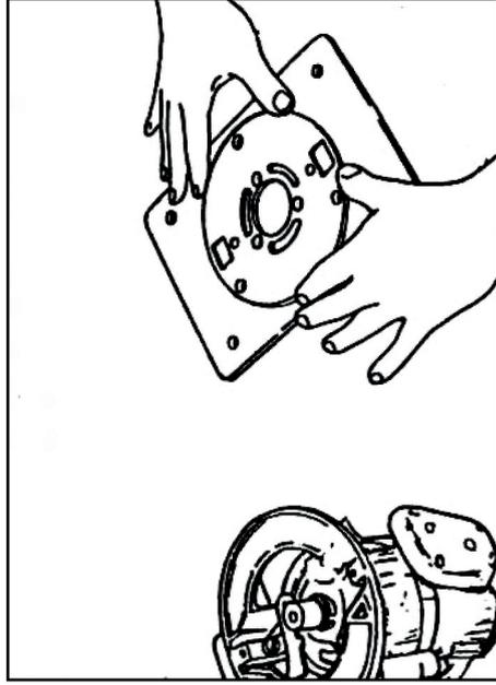
**Fig. 1** Remove the base plate from the router (Make sure power is disconnected prior to installing router or removing base plate) and align the table plate hole to the router base plate hole.
