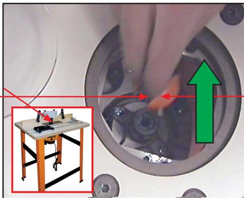
From the table top, extract the cutter to be replaced...
