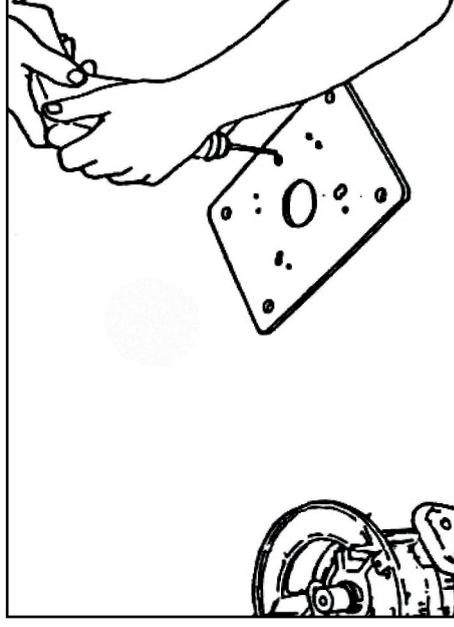
**Fig. 3** Drill mounting holes into the table plate and countersink or counter bore the top side of table plate so the head mounting screws are slightly below its surface.
