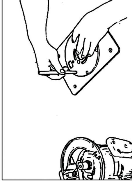
**Fig. 2** Use router base plate as a template to mark the location of each mounting hole onto the table plate.
