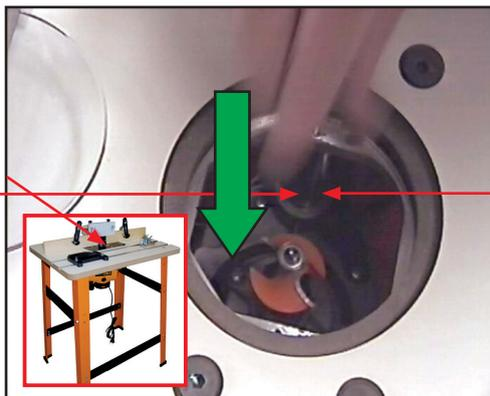
... and insert the new one, making sure that the stem is properly clamped by the gripper.
