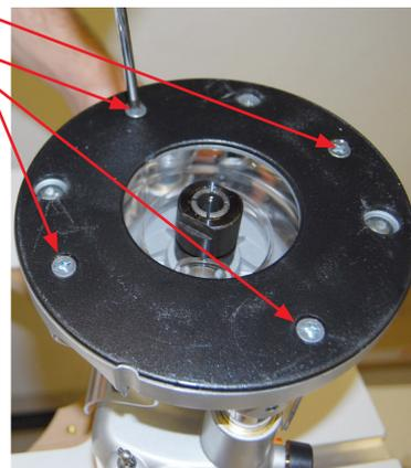
With a suitable screwdriver, remove the four screws as shown in the figure
