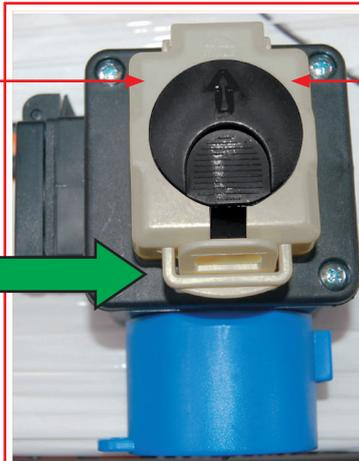
If the connection panel of the machine to the mains is not visible from the place where the machine is installed, to avoid accidental start-ups it is recommended to **add a lock to the switch.**
